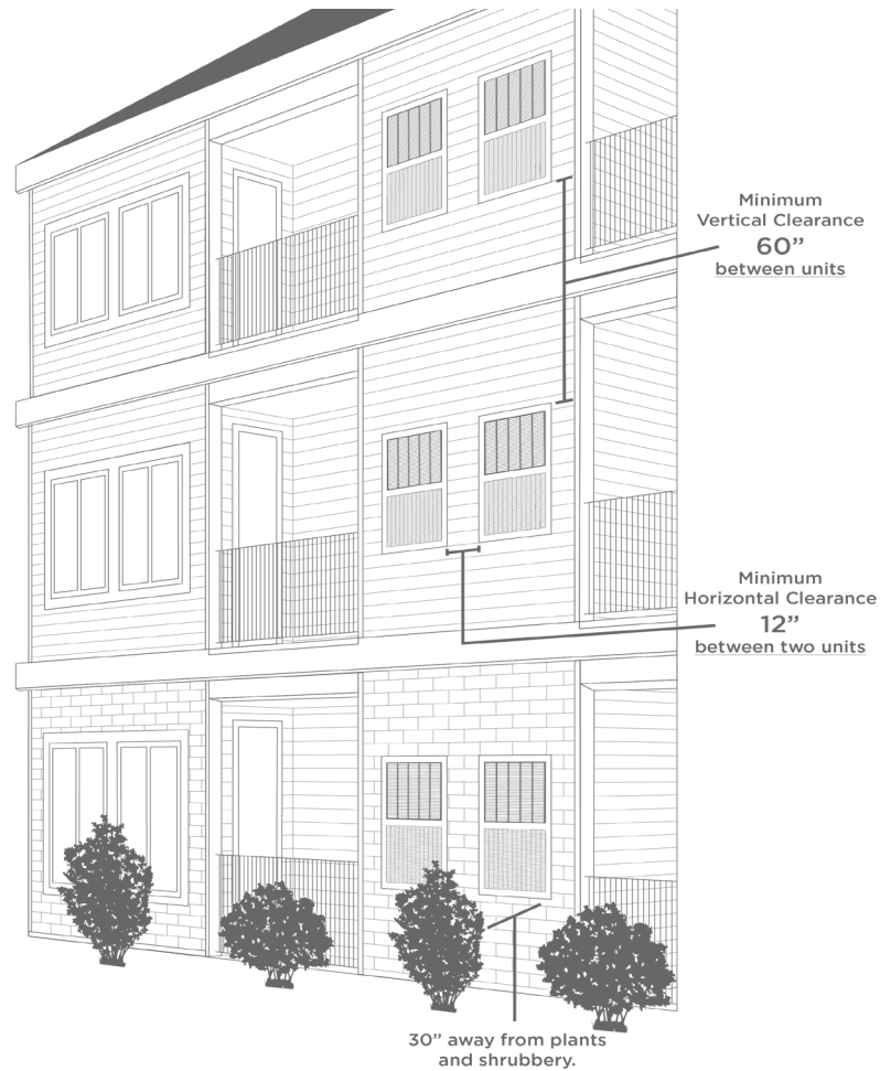
Fig 4: Recommended external clearances
